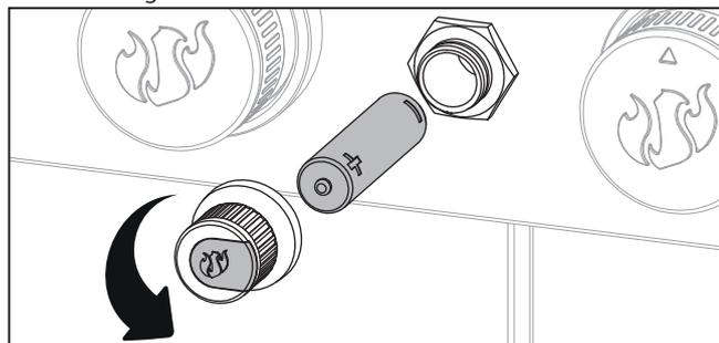
1. Twist the ignition button anticlockwise until it detaches.
