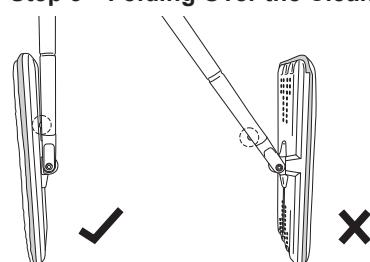
The cleaning foot (3) can only be folded over in one direction.
