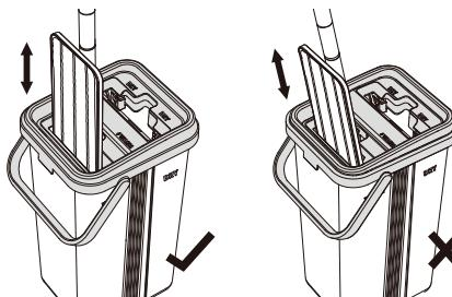
Place the cleaning foot (3) in the slot on the wringing attachment (7) labelled **DRY**. Move it back and forth several times until the desired level of moisture of the cleaning cloth (4) has been achieved.
