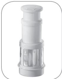
The sieve insert and plunger turn the mixing container into a juicer: The sieve insert filters out all solid elements such as pips and stems from the juice. You can use the plunger to feed in more ingredients during preparation.
