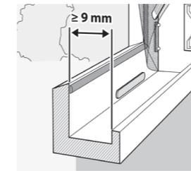
**Please Note!** The window frame must be at least 9 mm deep to allow the anti-pollen window mesh to be attached properly.
